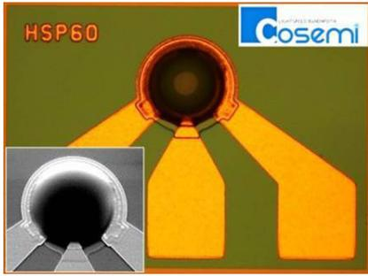
InkOrmo microlens printed on pre-patterned substrate, diameter of 100  $\mu\text{m}$  (Printed at EPFL, Courtesy of Cosemi Technologies Inc., USA)
