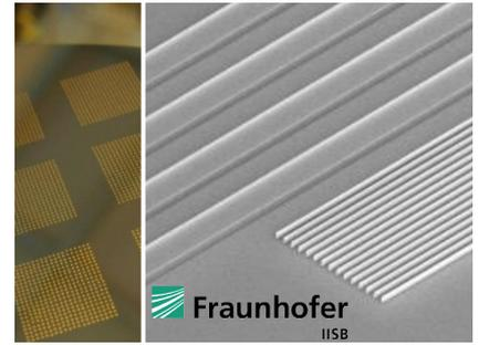
Left: Inkjet dispensed droplets. Right: subsequent imprinted submicrometer lines. (Courtesy of Fraunhofer IISB, Germany, 5)
