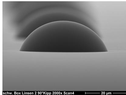
SEM pictures of cured InkEpo lens with  $\varnothing$  45  $\mu\text{m}$ , 10 drops per lenses on surface-treated glass slides. (Courtesy of EPFL, Switzerland)
