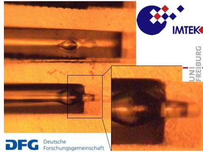
Inkjet-printed waveguide with 100  $\mu\text{m}$  core and 300  $\mu\text{m}$  cladding. (Courtesy of IMTEK, Germany, 2)
