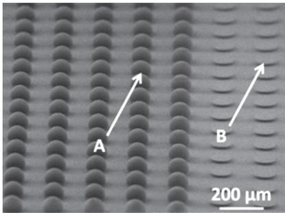
Array of InkEpo microlenses on 100  $\mu\text{m}$  wide Si platforms (A) lenses on a platform, (B) empty platforms. (Courtesy of EPFL, Switzerland)
