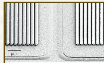
Slanted gratings in OrmoStamp® fabricated by replication (Courtesy of NILT, Denmark)
