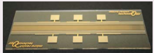
Microstructure array fabricated by multiple UV-photolithography and electroplating steps (Courtesy of Fritz-Haber-Institute, Berlin, Germany)
