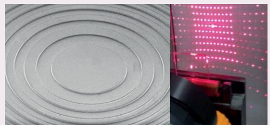
UV-Replication process done in cooperation with the Fraunhofer Heinrich-Hertz-Institute: 4"-Silicon master wafers with Fresnel Zone plates have been replicated into OrmoStamp® and OrmoComp®.
