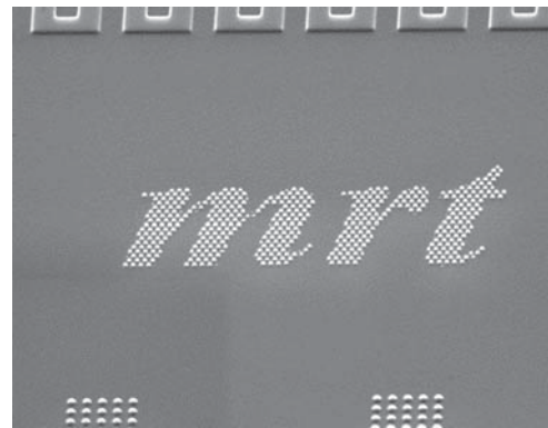
Imprinted with a Cr/Ni-coated OrmoStamp® stamp in mr-BioNIL100_SF_XP on a PET substrate, structure height of 180 nm and diameters of pillars of 400nm (small array in front) and 120 nm for logo
