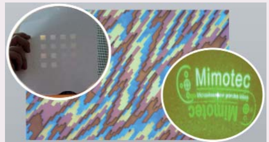
UV-NIL & LiGA process developed in cooperation with Mimotec SA : 4"-Silicon master replicated into UV-PDMS, OrmoStamp®, mr-NIL 6000E and electroplated into Nickel elements.
