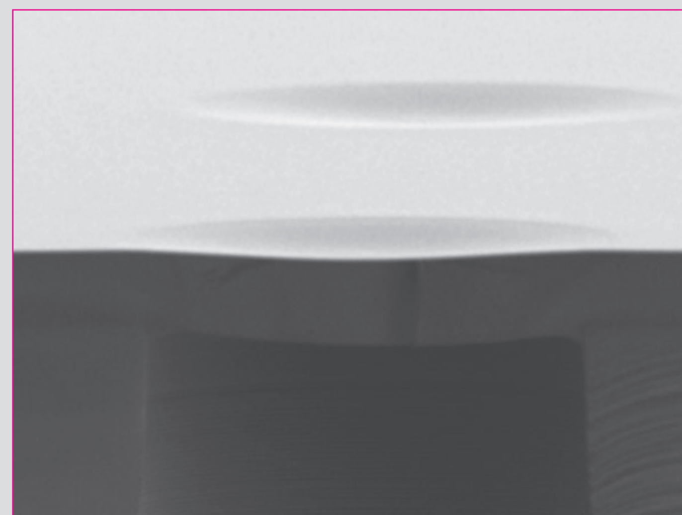
MX5000, Tenting over via-hole
