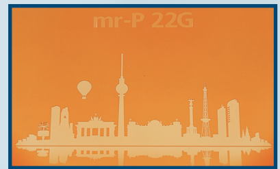
Greyscale pattern in mr-P 22G by Direct Write Lithography @ \lambda = 405 \text{ nm} with DWL 66+ 1)
