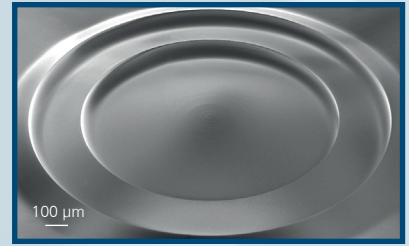
103 \mu\text{m} high, 2 mm diameter Fresnel lens 1) (DWL66+)
