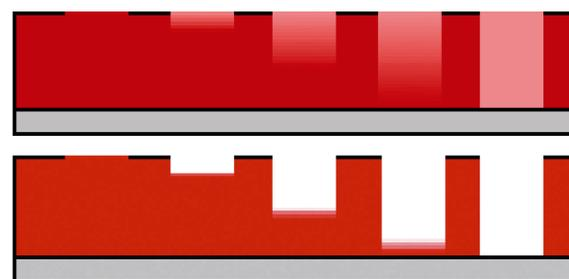
Figure 4 Top: Grayscale exposure of thicker resist films (FT ≥ 5 μm); Bottom: resist pattern after development.
