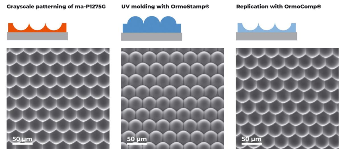
Figure 9: Pattern transfer of grayscale structures in ma-P 1275G by UV moulding with OrmoStamp® (left) to form a working stamp (center) and subsequently with OrmoComp® to form final concave lens structures (right).
