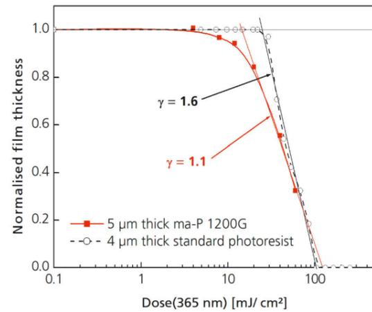
Figure 5: Contrast curves of 5 μm thick ma-P 1200G and of a 4 μm thick standard positive photoresist
