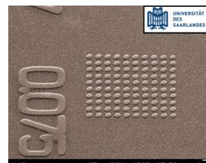
98 nm SiC dots 70 nm thick, after ICP
