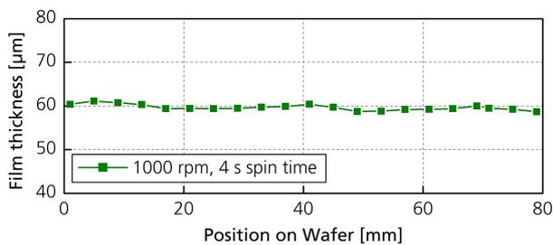
**Fig. 7.** Top: photograph of a 4" Si wafer coated with a 60  $\mu\text{m}$  thick ma-P 1275G film after spin-coating (1000 rpm, 4 s spin time) and edge bead removal. Bottom: Measured film thickness across the wafer after the softbake.
