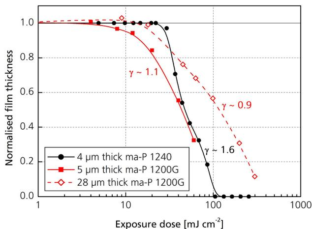
**Fig. 10.** Contrast curves of 5 µm and 28 µm thick ma-P 1200G and of 4 µm thick standard positive photoresist ma-P 1200 after mask aligner broadband exposure and development in 0.26N TMAH (ma-P 1200G) and 0.15N NaOH (ma-P 1200), respectively.
