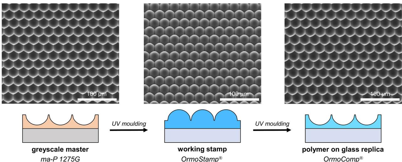
**Fig. 13.** Pattern transfer of greyscale structures in ma-P 1275G, concave lenses, by UV moulding with OrmoStamp® to form a working stamp and subsequently with OrmoComp® to form final concave lens structures.
