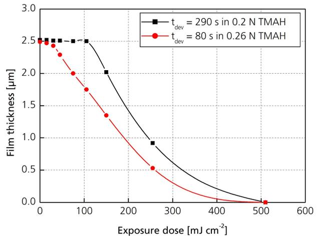
**Fig. 11.** Response curves of 2.5 µm thick ma-P 1225G with monochromatic 365 nm LED exposure ( $I = 150 \text{ mW cm}^{-2}$ ), development in 0.2N and 0.26N TMAH.
