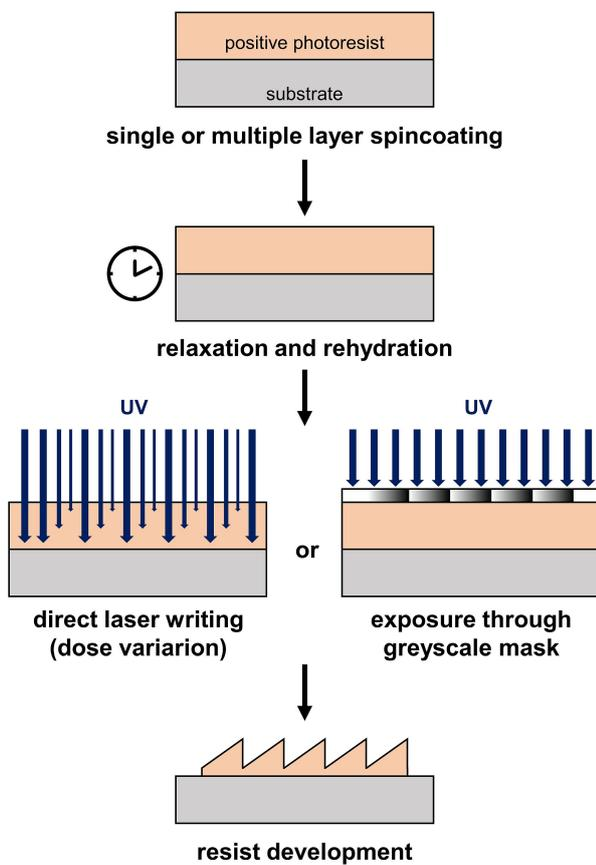
**Fig. 2.** Greyscale lithography process using a positive greyscale resist and different options for UV exposure: direct laser writing (left) and mask aligner exposure using a greyscale mask (right).
