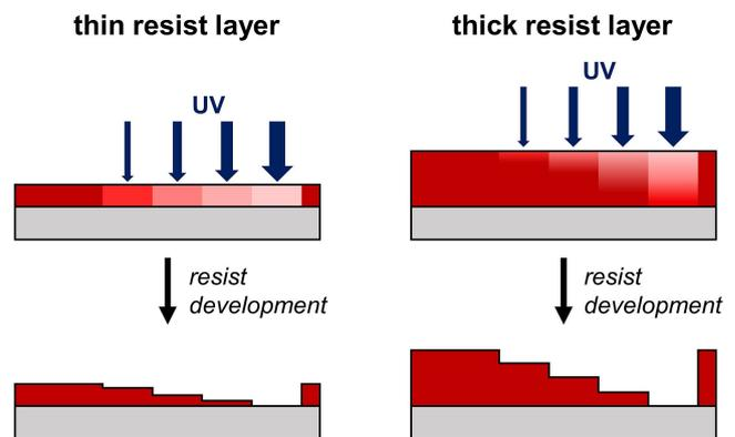
**Fig. 5.** Greyscale exposure of thin (FT ≤ 5 μm) and thick (FT > 5 μm) resist films.
