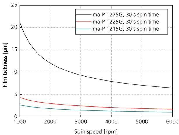
**Fig. 6.** Film thickness obtained with different resists of the ma-P 1200G series by spin coating with 30 s spin time.
