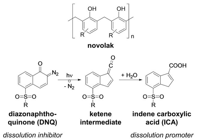
**Fig. 3.** Structure of novolak used as polymeric binder in positive photoresists (top) and photoreaction of DNQ photoactive compound during exposure of the resist (bottom).
