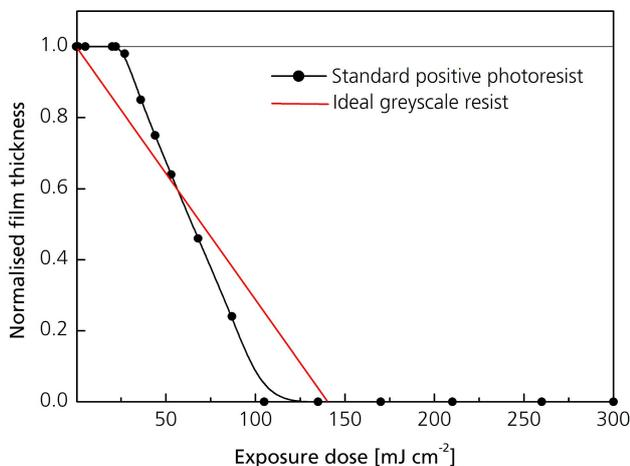
**Fig. 4.** Response curves (normalised film thickness FT/ FT<sub>0</sub> after development vs. exposure dose) of a standard binary positive photoresist and an ideal greyscale resist.
