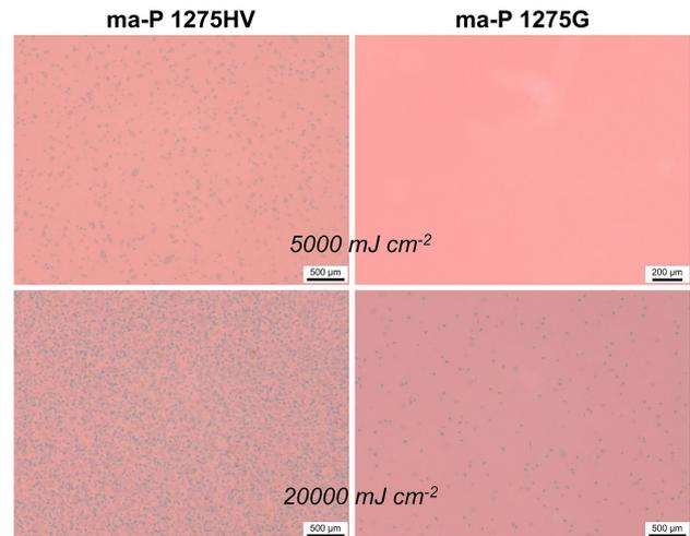
**Fig. 8.** Optical microscope image of bubble formation due to resist outgassing in  $\sim 60 \mu\text{m}$  thick films of ma-P 1275HV (left) and ma-P 1275G (right) after LED exposure at 410 nm ( $I = 275 \text{ mW cm}^{-2}$ ). Exposure dose:  $5000 \text{ mJ cm}^{-2}$  (upper row) and  $20000 \text{ mJ cm}^{-2}$  (bottom row).
