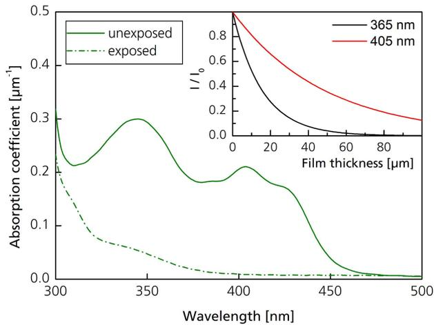
**Fig. 9.** UV/vis absorption spectra of an unexposed and exposed ma-P 1200G resist film, measured on a 1 x 2.5 cm<sup>2</sup> quartz substrate in 4 µm film thickness (absorbance normalised to 1 µm film thickness). Inset: Resulting light attenuation at 365 nm and 405 nm calculated using Lambert-Beer's law.
