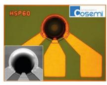
InkOrmo microlens printed on pre-patterned substrate, diameter of 100  $\mu$ m (Printed at EPFL, Courtesy of Cosemi Technologies Inc., USA)
