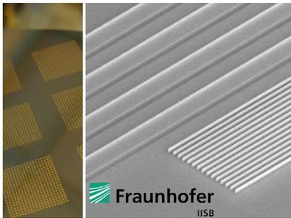
Left: Inkjet dispensed droplets. Right: subsequent imprinted submicrometer lines. (Courtesy of Fraunhofer IISB, Germany, 5)
