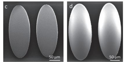
SEM images of (c) SU-8 platforms and (d) the corresponding lenses after performing the IJP of the InkEpo onto the platforms. (Courtesy of EPFL, Switzerland)
