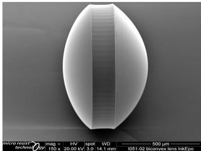
Biconvex InkEpo microlens made by a combination of inkjet dispensing and UV replication
