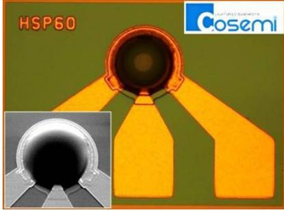
InkOrmo microlens printed on pre-patterned substrate, diameter of 100 μm (Printed at EPFL, Courtesy of Cosemi Technologies Inc., USA)
