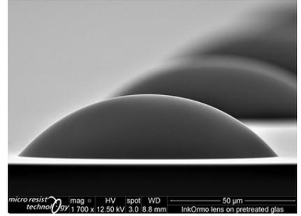
Exemplary InkOrmo microlens on pretreated glass substrate (100 μm diameter)
