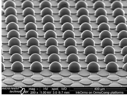
InkOrmo microlens array on OrmoComp platforms with 100 μm diameter as a confining pattern (Courtesy of EPFL/Switzerland)
