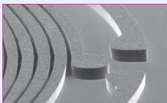
Electroformed Nickel coil - 30 µm
