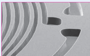
UV imaging of a 30 µm thick micro coil
