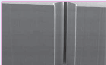
Preparation of a 1000 µm thick resist layer
