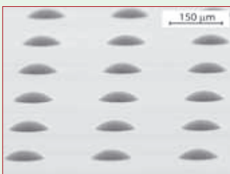
SEM of replicated microlenses in sol-gel material (CSEM)
