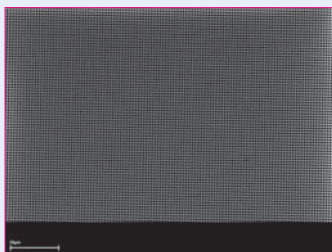
Imprinted 800 nm squares, 1200 nm pitch, large-area imprint (Courtesy of Profactor)
