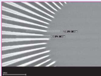
Imprinted lines, sub-30 nm resolution (Courtesy of AMO)
