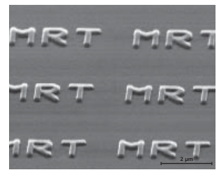
mr-UVCur06 structures (32nd imprint done with an OrmoStamp mould)
