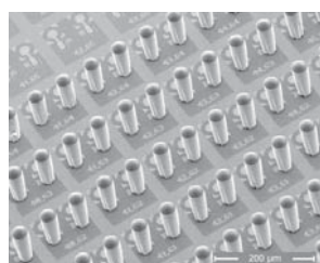
Replicated refractive microlenses on a VCSEL wafer substrate (Courtesy of Avalon)
