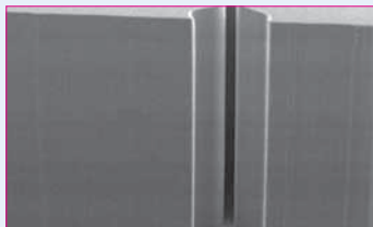
Preparation of a 1000 µm thick resist layer
