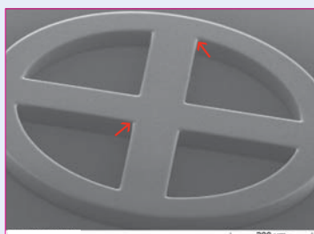
No microcracks on critical spots
